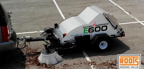
Now includes four 24V Lithium-ion rechargeable batteries as standard
